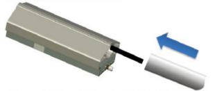
Power cable through the pole and the pole fix in luminaire's holder.
